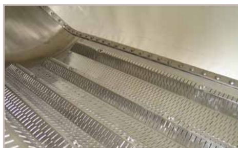
connected draining channels, electropolished
